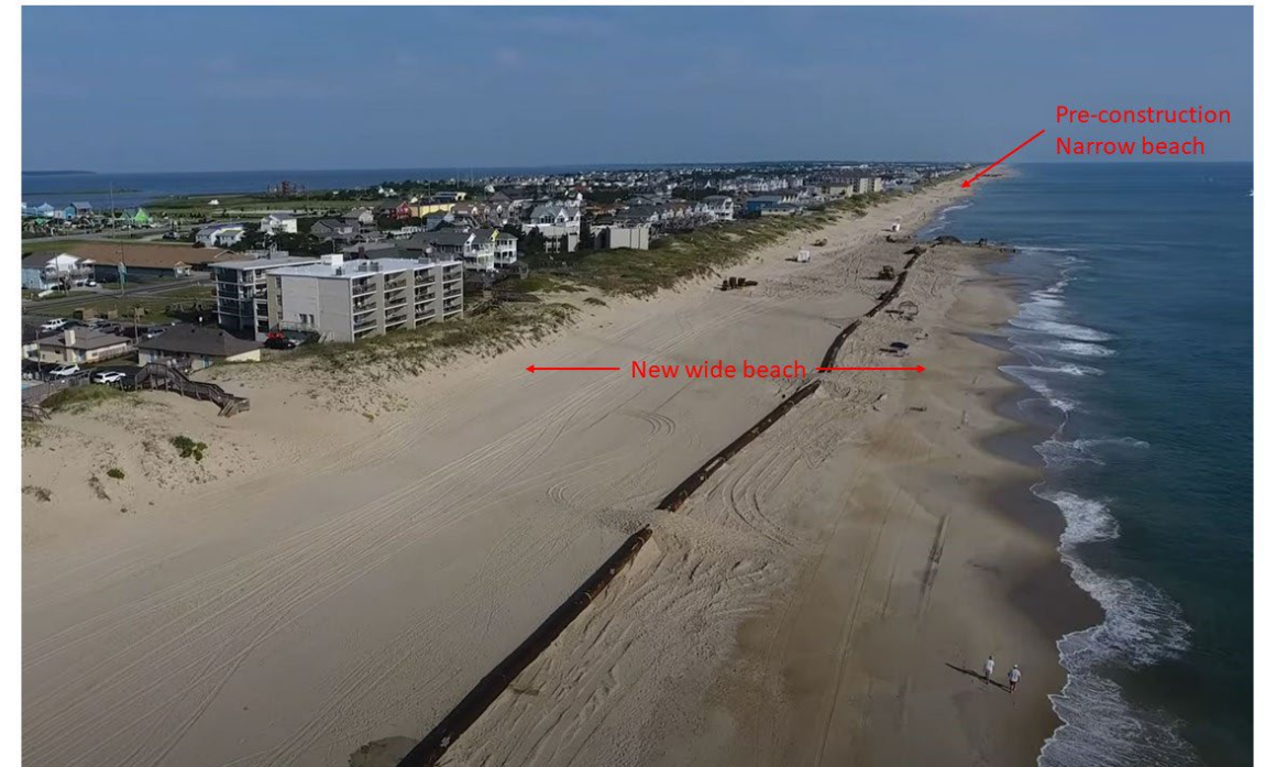
Example of an adaptation measure of beach renourishment being implemented
