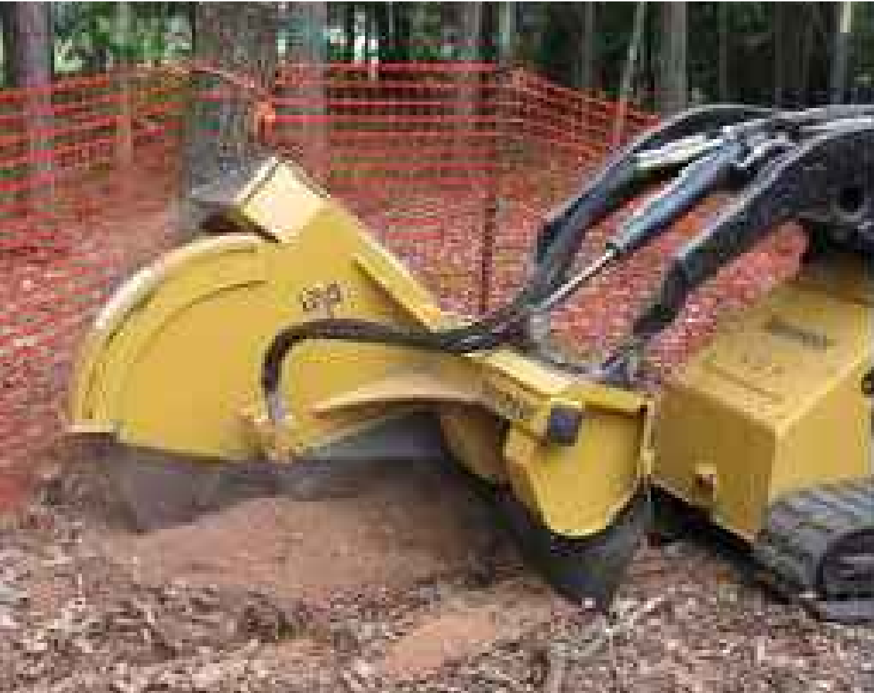
CONTRACTOR TO USE DOSKO OR VERMEER MECHANICAL ROOT PRUNER EQUIPMENT WHEN WITHIN CRITICAL ROOT ZONE OR TREE PROTECTION AREA FOR INSTALLATION OF 4" CONDUITS FOR ELECTRICAL, CABLE, TELECOMMUNICATIONS AND IRRIGATION SERVICES
